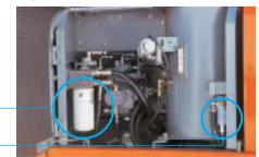
**Engine Oil Filter and Water Separator Positioned for Easy Checking from Ground**
